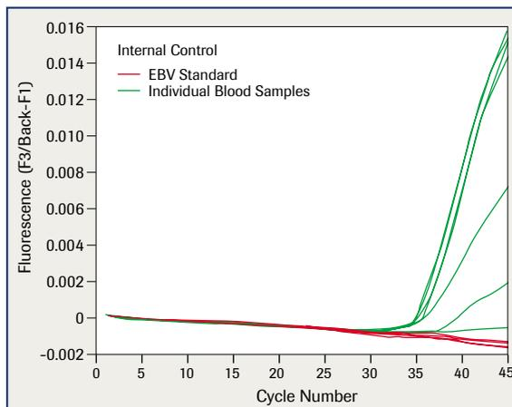
Figure 2: LightCycler PCR amplification curves of the Internal Control (IC). IC is only present in the individual samples (green) not in the standards (red).
