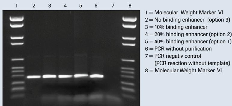
**Figure 2: Agarose gel electrophoresis and ethidium bromide staining of 341 bp PCR products.**
