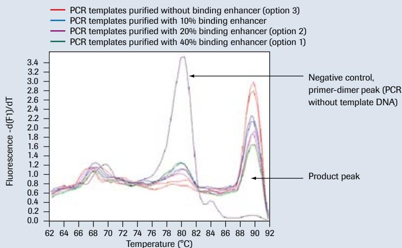
**Figure 3: Melting curve analysis after the last PCR cycle using a LightCycler® 1.5 Instrument.**
