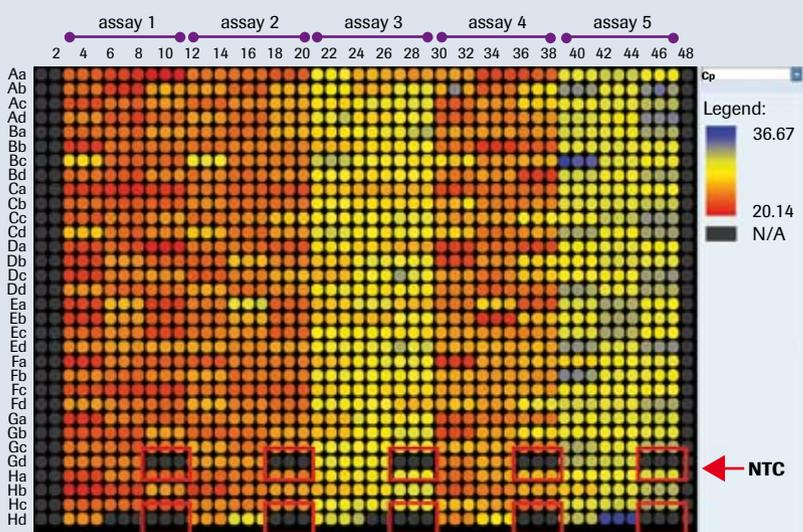
**Figure 4: Heatmap chart of the LightCycler® 1536 Software.** Shown are the Cp values of five different assays with 96 cDNA samples including two no-template control samples (NTC) on one plate. The Cp values of the samples are displayed as a continuous spectrum from blue (highest Cp) to red (lowest Cp; see legend).
