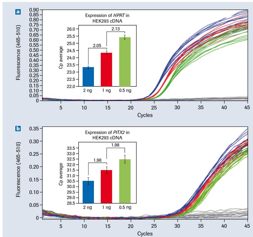
**Figure 2: Comparing amplification curves of genes with different expression levels.** Expression levels of *HPRT* and *PITX2* in HEK293 cells were measured with the LightCycler® 1536 Instrument using a dilution series of cDNA (2 ng in blue, 1 ng in red, 0.5 ng in green and NTC in grey). The determined dilution factor corresponded well with the theoretical dilution factor of 2. Measurements were performed in 12 replicates.
