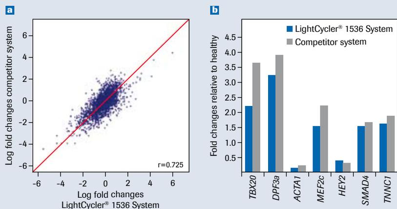
**Figure 5: Comparison of gene expression fold changes between the LightCycler® 1536 System and a competitor real-time PCR system (384-well format).** Fold changes are normalized to *HPRT* and relative to healthy individuals. **(a)** Dot plot with Pearson correlation coefficient ( $r=0.725$ ) of 40 genes and 71 samples. **(b)** Comparison of a subset of transcripts relevant to the heart in a group of individuals with tetralogy of Fallot individuals.
