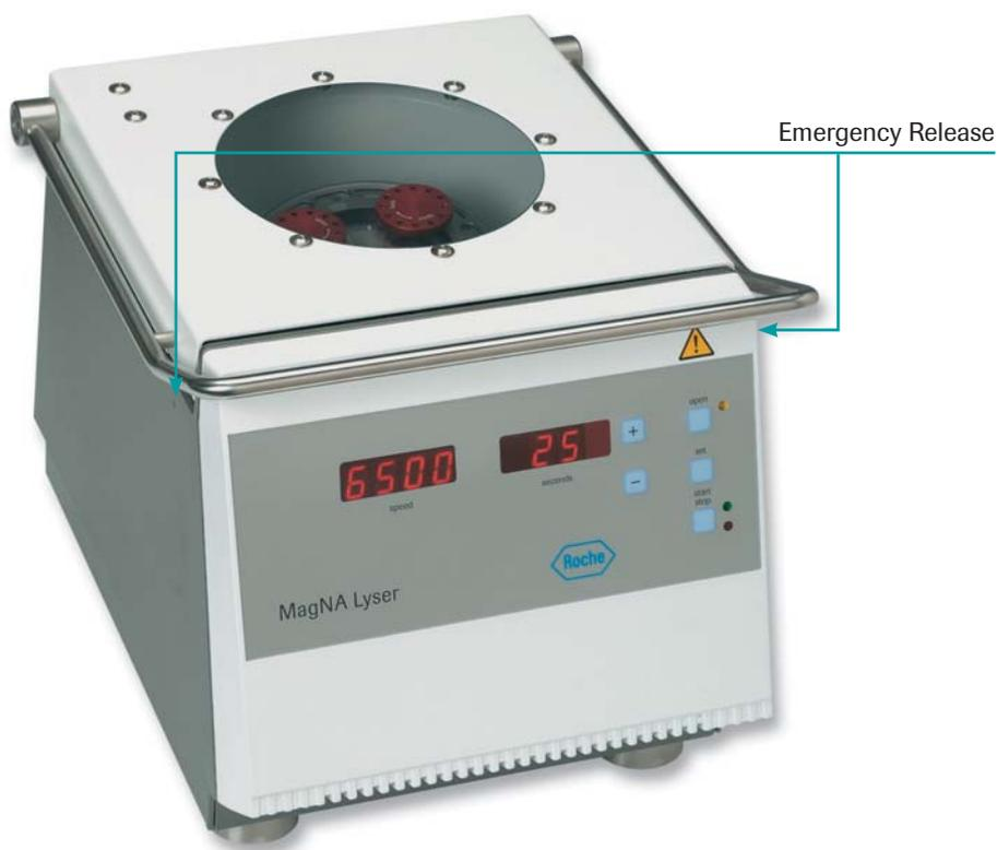
Figure 11: Emergency Interlock Override
