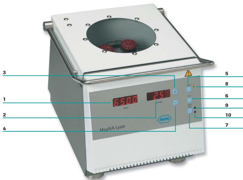
Figure 2: MagNA Lyser Instrument; view from the front
