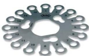
3. Two MagNA Lyser Rotors [If necessary, you may order additional rotors (Cat. No. 03 359 093 001).] (Figure 1c)
