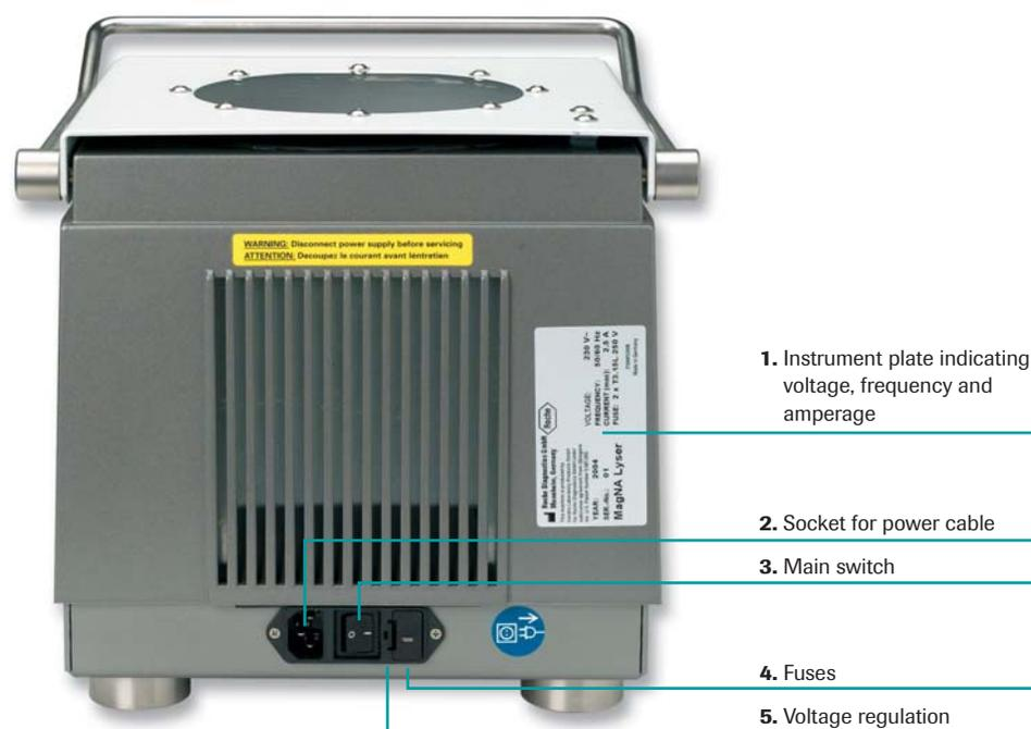
Figure 3: MagNA Lyser Instrument, view from the rear
